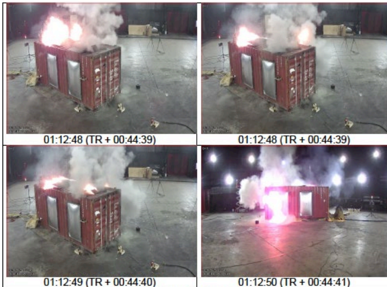
Figure 85 – Deflagration images from Test 2.
